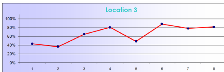
Figure 8: Example of output of the KPI module-evolution of the percentage utilization of storage location 3 during 8 h.
